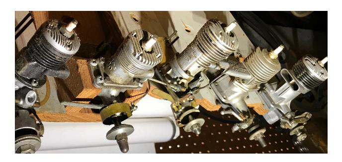
He made his own ingenious magneto ignition systems for the engines with spark plugs as can be seen in these photos.
