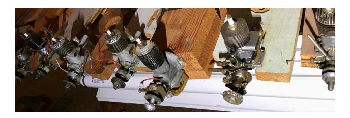
The compression-ignition (no spark plug, no glow plug) powerplants ran on a mixture of ether, kerosene and castor oil or 30wt engine oil, - approximately one third part each. This was
